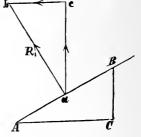
Let  $R_1$  be the reaction of the groove at any point a. Construct the triangle abcequal in every respect to ABC.
